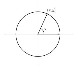
If  $\alpha < 0$ , rotate the ray by  $|\alpha|$  radians in the clockwise direction.
