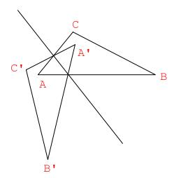
4. Glide reflection—reflection across a specified line followed by a translation parallel to that line by a specified amount. We can indicate the glide reflection by drawing the line and drawing a parallel vector. Remember that a reflection is a special case of a glide reflection in which the translation amount is zero.
