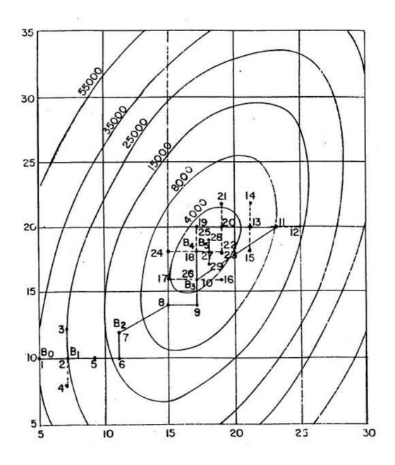
Figure 2: Hooke and Jeeves Pattern Search: Graphical Illustration of the Example
