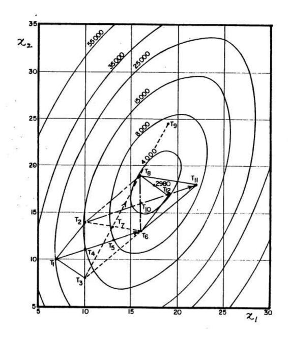
Figure 1: Nelder-Mead Simplex Method: Graphical Illustration of the Example
