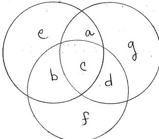
(a) Extend the code  $\{a,b,c,d\} = \{0,1,0,1\}$  to a seven-bit Hamming Code by filling in the Venn diagram corresponding to the figure above. (2pts)
