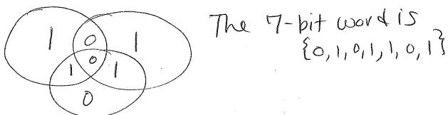
(b) At most one bit is in error in the Hamming code word  $\{a, b, c, d, e, f, g\} = \{0, 0, 1, 1, 1, 1, 1\}$ . Determine whether this word is correct, or if it is incorrect, correct the code. (3pts)
