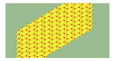
Tiling by quadrilaterals made with SketchUp. Adjacent quadrilateral is obtained by rotation about midpoint of shared edge. Then pairs of quadrilaterals are translated.
