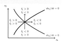
The point where both null clines in the picture intersect is a point equilibrium or critical point, which we call  $\hat{\mathbf{x}}$ . We can use the graph to determine the signs of the entries in the Jacobi matrix
