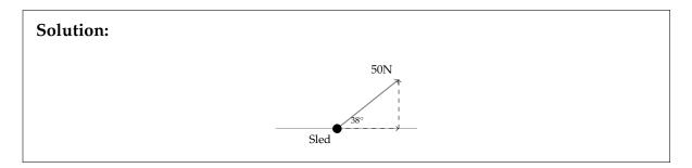
The horizontal and vertical components of the 50N force are given by the dashed lines in the diagram above. We see from the figure that the horizontal force is given by  $50 \cos(38^\circ)$  while the vertical force is given by  $50 \sin(38^\circ)$ . Therefore, the 50N force can be written in component for as  $50 \cos(38^\circ)\mathbf{i} + 50 \sin(38^\circ)\mathbf{j}$ .
