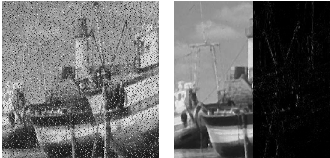
Figure 9: The Boat images in 256 \times 256 cells, with (left) a random-valued impulse noise of 20% possibility and (right) restored by the hybrid algorithm. For the right figure, the right half is adjusted to show the absolute distance between the original image and the restored one.
