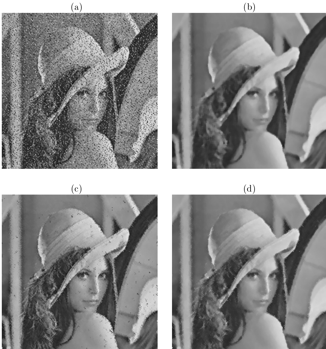
Figure 1: The Lena images in 256 \times 256 cells, with (a) random-valued impulse noise of probability 20%, and restored images by the running (b) median, (c) CWM, and (d) PCWM filters. The window size is 5 \times 5 for the median filters.
