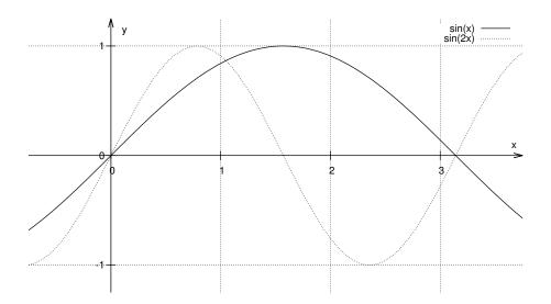
The graph of  $\sin(2x)$  is obtained by compressing the graph of  $\sin(x)$  by a factor of 2. Thus, a tangent line to the graph of  $\sin(2x)$  at a point  $(a/2, \sin(a))$  will be twice as steep as the corresponding tangent line to the graph of  $\sin(x)$  at the corresponding point  $(a, \sin(a))$ .
