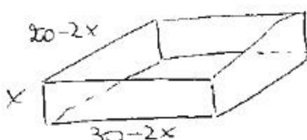
$$\begin{aligned} \text{Volume } V(x) &= x \cdot (20-2x)(30-2x) \\ &= 4x(10-x)(15-x) \end{aligned}$$
