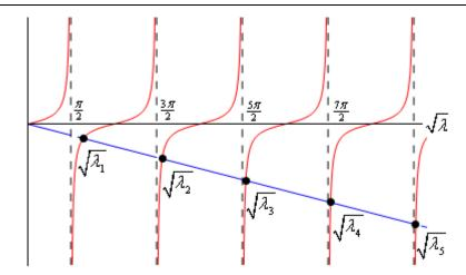
So, eigenvalues for this case will occur where the two curves intersect. We've shown the first five on the graph and again what is showing on the graph is really the square root of the actual eigenvalue as we've noted.
