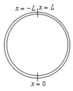
We will measure x as positive if we move to the right and negative if we move to the left of x = 0. This means that at the top of the ring we'll meet where x = L (if we move to the right) and x = -L (if we move to the left). By doing this we can consider this ring to be a bar of length 2L and the heat equation that we <u>developed</u> earlier in this chapter will still hold.
