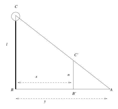
Solution. We draw two right triangles so that l = 20 m is the height of the light and n = 2 m is the height of the man. These lengths are fixed, so dn/dt = dl/dt = 0. The function x = x(t) gives the distance of the man from the light and we are told that dx/dt = 0.9 m/s. We do not want to substitute x = 15 yet as this would not allow us to use the information that x is changing.
